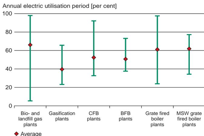
Comparison of the utilisation factor for the different technologies, based on operational data for 24 months
