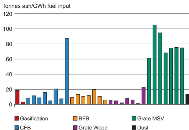
Amount of ash produced in the plants shown in metric tonnes pr. GWh fuel input. Ash weight includes any water mixed into the ashes.
