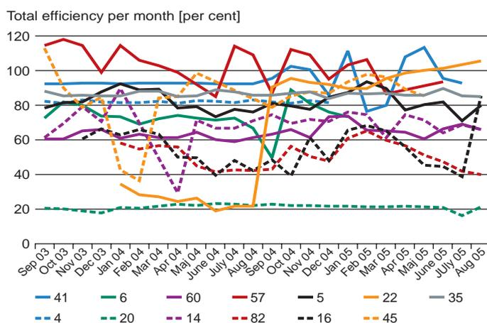
Total of heat and electric efficiencies for 13 grate fired biomass CHP systems. Operational figures are monthly data shown for 24 months, September 2003 to August 2005
