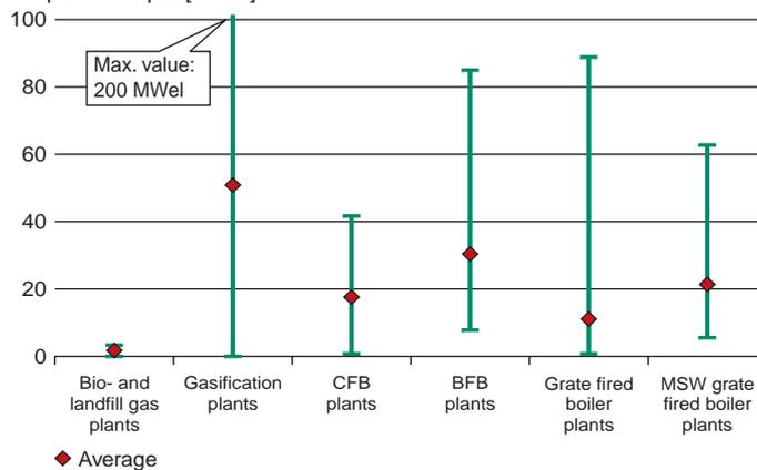
Comparison of the size, shown as min, max and average net electric capacity, for the different technologies.
