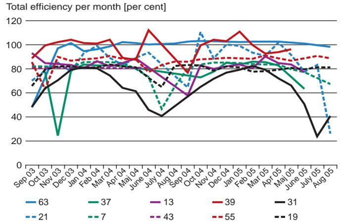
Total of heat and electric efficiencies for 10 BFB biomass CHP system. Operational figures are monthly data shown for 24 months, September 2003 to August 2005.
