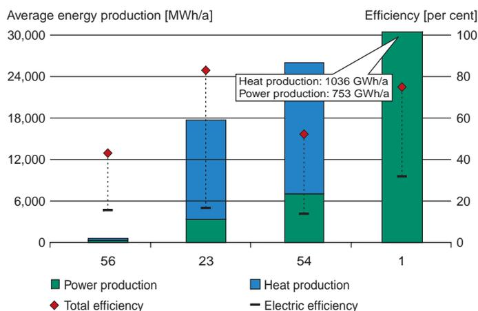
Operational efficiencies for 4 biomass gasifier CHP systems compared to the size of the plant shown as the annual production of electricity and heat. Operational figures are average values for 24 months, September 2003 to August 2005.
