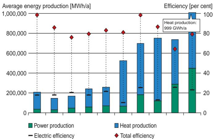
Operational efficiencies for 10 BFB biomass CHP systems compared to the size of the plant shown as the annual production of electricity and heat. Operational figures are average values for 24 months, September 2003 to August 2005.
