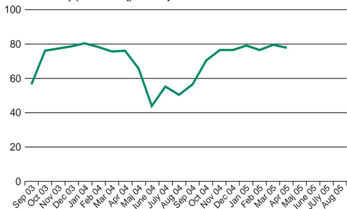
Total of heat and electric efficiencies for the dust-fired CHP plant. Figures are monthly data shown for 24 months, September 2003 to August 2005.
