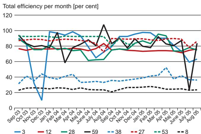
Total of heat and electric efficiencies for 8 MSW grate fired biomass CHP systems. Operational figures are monthly data shown for 24 months, September 2003 to August 2005.
