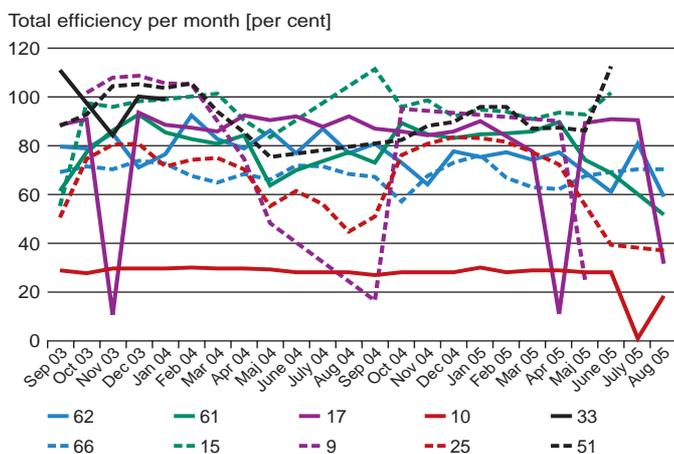
Total of heat and electric efficiencies for 10 CFB biomass CHP systems. Operational figures are monthly data shown for 24 months, September 2003 to August 2005
