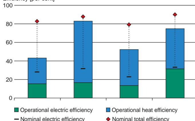
Nominal and operational efficiencies for 4 biomass gasification CHP systems. Operational figures are average values for 24 months, September 2003 to August 2005.
