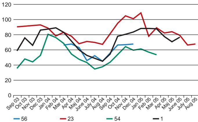
Total of heat and electric efficiencies for 4 biomass gasifier CHP systems. Operational figures are monthly data shown for 24 months, September 2003 to August 2005.
