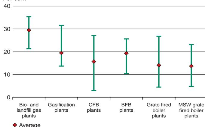
Comparison of min, max and average electric efficiency for the different technologies based on operational performance data for 24 months.
