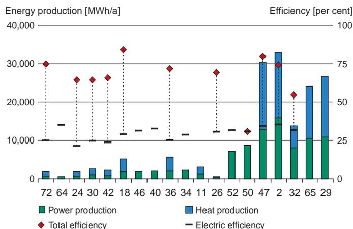
Operational efficiencies for 19 biogas and landfill gas CHP systems compared to the size of the plant shown as the annual production of electricity and heat. Operational figures are average values for 24 months, September 2003 to August 2005.
