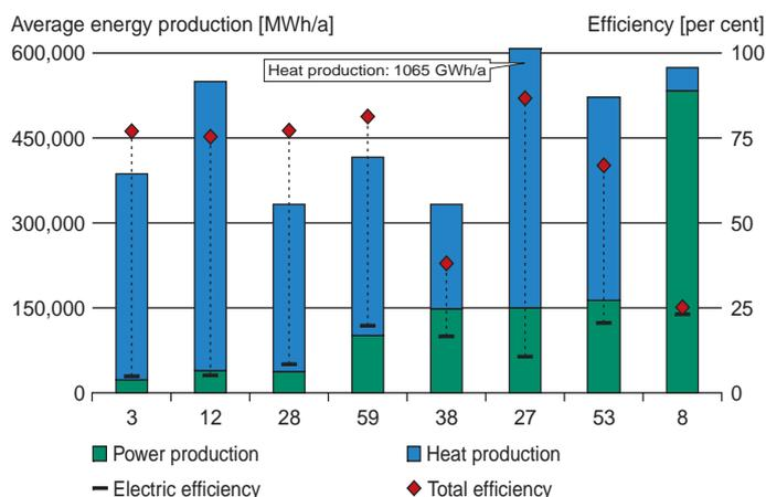
Operational efficiencies for 8 grate fired biomass CHP systems compared to the size of the plant shown as the annual production of electricity and heat. Operational figures are average values for 24 months, September 2003 to August 2005.
