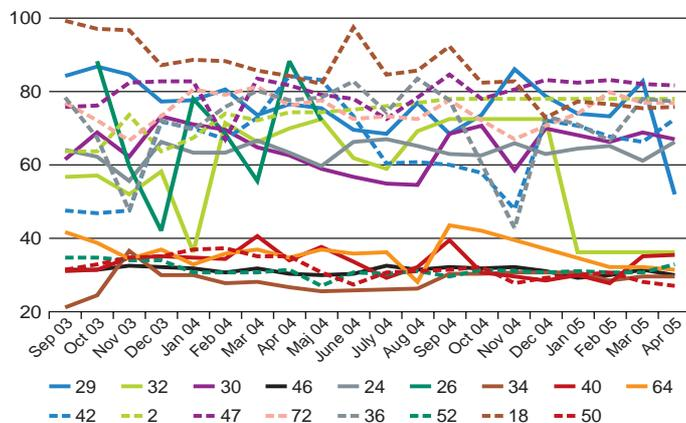
Total of heat and electric efficiencies for 19 biogas and landfill gas CHP systems. Operational figures are monthly data shown for 24 months, September 2003 to August 2005.
