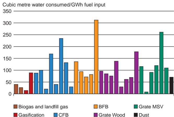
Consumption of water in the plants shown in m<sup>3</sup> pr. GWh fuel input.
