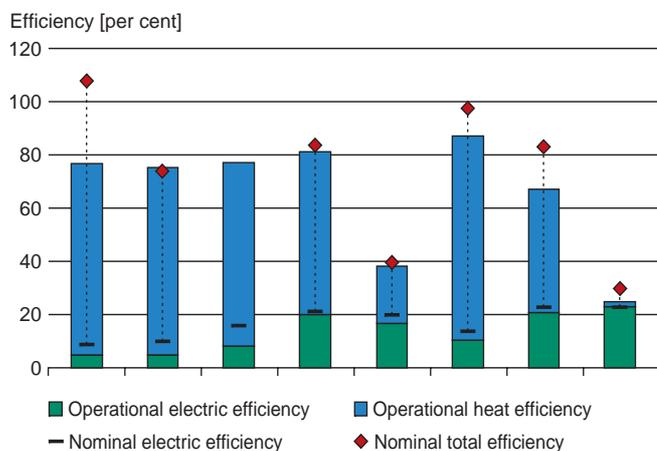
Nominal and operational efficiencies for 8 MSW grate fired biomass CHP systems. Operational figures are average values for 24 months, September 2003 to August 2005.
