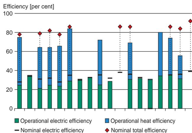
Nominal and operational efficiencies for 18 biogas and landfill CHP systems. Operational figures are average values for 24 months, September 2003 to August 2005.
