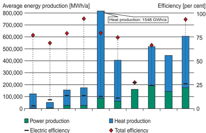
Operational efficiencies for 10 CFB biomass CHP systems compared to the size of the plant shown as the annual production of electricity and heat. Operational figures are average values for 24 months, September 2003 to August 2005.
