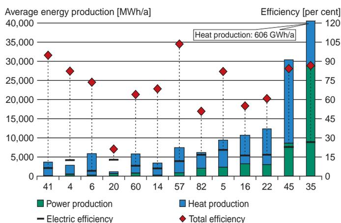
Operational efficiencies for 13 grate fired biomass CHP systems compared to the size of the plant shown as the annual production of electricity and heat. Operational figures are average values for 24 months, September 2003 to August 2005.
